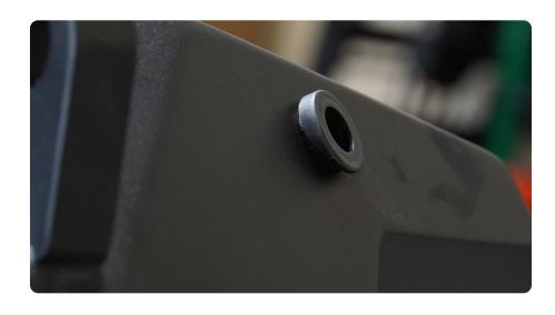
**STEP 14** | Install trailer wiring plug from the front side of the bumper until it snaps into place. Connect to harness.
