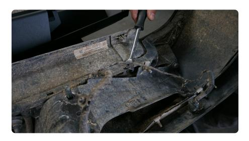
**STEP 7** Once the wire harness if free from the bumper, disconnect the two license plate lights by depressing the tab on the plug and pulling away from the light.
