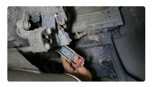
**STEP 3** Disconnect the wiring from frame releasing a trim clip tool so that the wiring is free.
