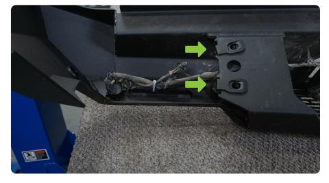
STEP 17 | If the vehicle is equipped with dual exit exhaust, remove the two lower panels using a 10mm and #4 Allen bit.
