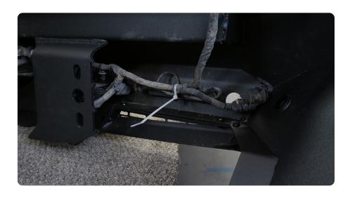
**STEP 16** | Take the M12 flat nuts, and slide them in place over the bumper mounting holes.
