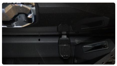
STEP 22 | Plug in the harness into the factory plugs that were removed in steps 1 & 2.
