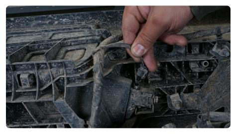
**STEP 8** Next, remove the sensors (if equipped). Do not unplug the sensors, rather, gently spread the two clips on each side of the sensor and pull the sensor back away from the bumper.
