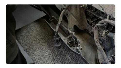
STEP 9 Remove the trailer plug. Using a flat head or trim clip tool, press in both sides of the metal retaining clip and push the plug out towards the front of the bumper.
