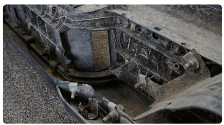
**STEP 11** Begin by feeding the wiring harness through the cavities of the bumper until sensors and light plugs align with their new holes.
