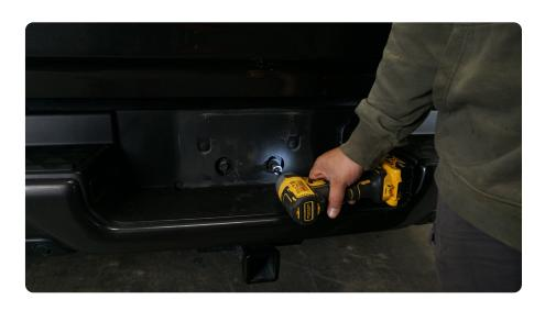
STEP 5 Using a 16mm socket or wrench, remove the (4) nuts (2 per side) to release the bumper.
