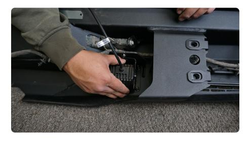
STEP 19 | With assistance to prevent injury or damage to the vehicle, lift the bumper to the truck and using the provided M12 hardware (bolt, flat washer and spring washer), loosely secure the bumper to the vehicle.
