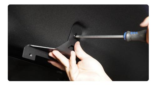
STEP 5 Using the provided M6 allen head bolts and washers, loosely install the lower bracket onto the molle panel.
