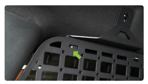
STEP 7 | Line up the panel so it is even around the window and secure all hardware until tight.
