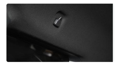
STEP 2 | Squeeze the top and bottom tabs together and pull towards you to remove the clip and the hanger.
