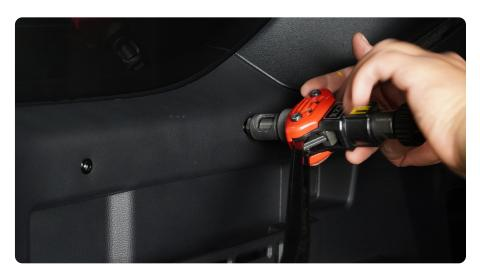
STEP 10 | With the nutserts in place reinstall the panel. If all the hardware is loosened, then adjusting the panel to align will be much easier.
