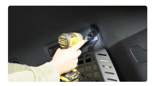
STEP 8 | Using the provided M6 hardware, secure the lower bracket to the aluminum spacers.
