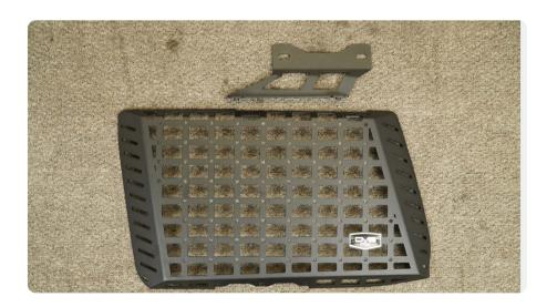
STEP 2 | Using the provided M6 hardware and #4 allen head, attach the bracket leaving it loose for adjustment.
