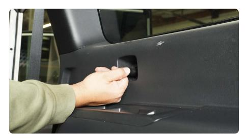
STEP 7 | Hold up the molle panel and using the factory hardware AND handle, secure the upper mount to the factory holes using a 10mm socket.
