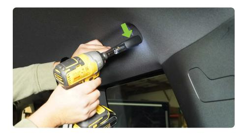
STEP 5 Using the trim pry tool, remove the plastic caps on the panel under the window. Using a 10mm remove the bolt inside this cover.
