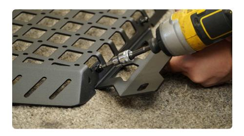
STEP 3 | Flip the panel over and using the M6 hardware and a #4 allen head, install the lower bracket as shown.
