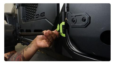
STEP 5 | Drill out the marked mounting holes using a small drill bit, working your way up to a 9/32" bit.
