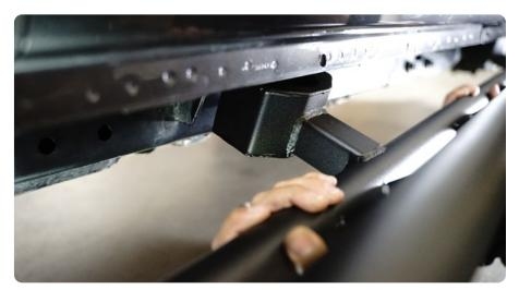
STEP 5 | When all hardware is loosely installed, finish securing all factory hardware using a 16mm and 18mm socket with a 10" extension.
