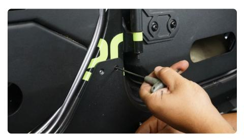
STEP  $8 \mid$  with the rock skins installed and the hardware secure, use a punch tool to mark the remaining mounting holes for drilling.
