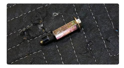
STEP 17 | Slide the nutsert tool with the nutsert into the mounting hole.
