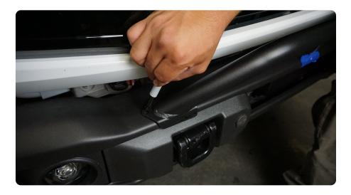
STEP 7 Use a 11/32nd drill bit to drill the (6) bull bar mounting hole into the bumper.
