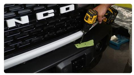
STEP 8 | Insert and secure the provided M8 rivnuts into the hole previously drilled into the bumper using a preferred rivnut tool(not included).
