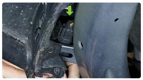
**STEP 15** | To gain better access to the plug, use a push pin tool to release the plug from the body.
