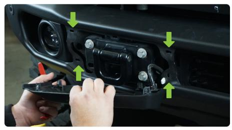
**STEP 13** | Disconnect cable from sensor on each plastic cover.
