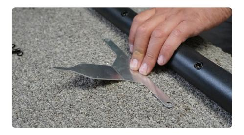
STEP 2 Attach the provided alignment tool to the bull bar using the provided M6 hardware. Use a #4 Allen tool to secure the M6 hardware.
