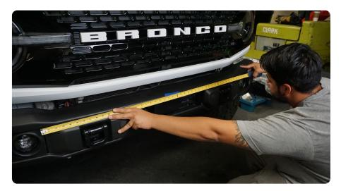
**STEP 5** | With the center of the bumper marked, hold the bull bar on the bumper using the alignment tool to center the bull bar.
