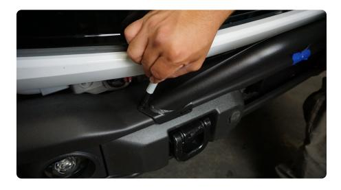
STEP 7 Use a 27/64ths drill bit to drill the (6) bull bar mounting hole into the bumper.
