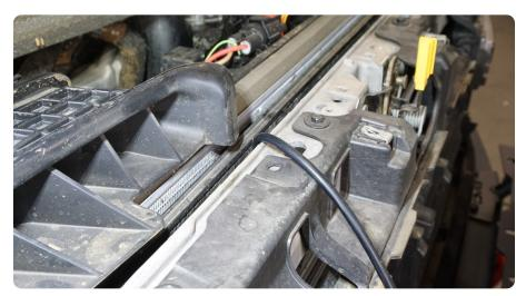
STEP 17 | Connect the provided front camera harness to the factory harness under the hood/ above the headlight.
