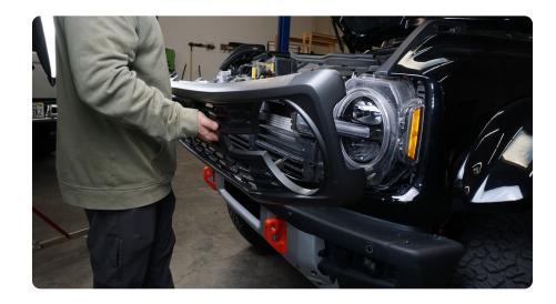
STEP 6 | Set the Grille on a covered work bench. Locate the (4) torx bolts that secure the front camera to the grille.
