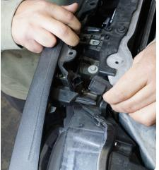
STEP 4 Disconnect the front camera and washer fluid hose on the passenger side.
