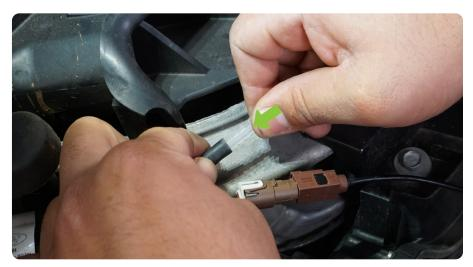
STEP 19 Cut the washer fluid hose coming from the front camera to length. Connect the provided hose to the factory washer hose.
