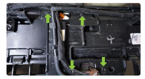
STEP 7 | With the camera and camera cover removed from the grille housing, disconnect the camera from the factory wiring harness.
