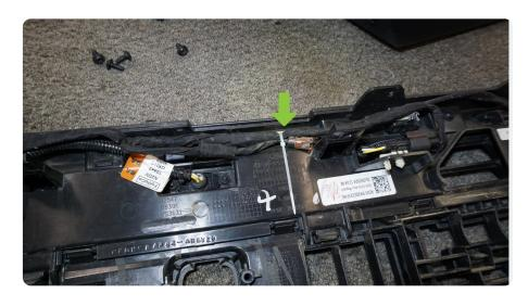
STEP 9 | Separate the front camera washer fluid nozzle and check valve from the factory washer fluid 90 degree hose.
