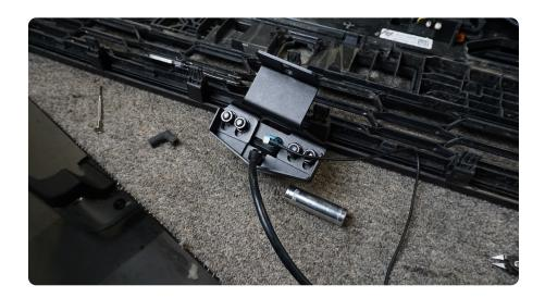
STEP 13 | Using a T45 torx tool, remove the factory bumper bolts above the factory recover hooks. (3 bolts per side)
