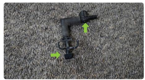
STEP 10 Using a small section of the provided washer fluid hose. Reinstall the washer fluid nozzle and check valve as shown.
