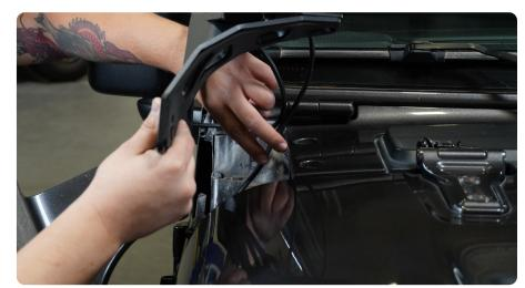
STEP 8 | Re-place the body panel and light bar bracket and secure the provided and factory hardware with a T-40 torx, #4, and #5 allen bit.
