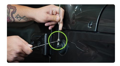
STEP 3 | Use a T40 torx bit to remove the three factory bolts on each side of the vehicle.
