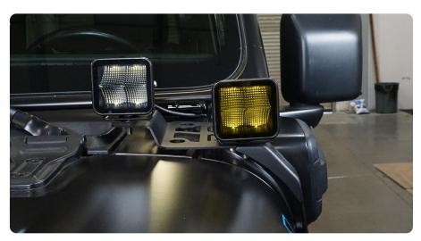
STEP 5 Using a T40 Torx bit and factory hardware, secure the DV8 A-Pillar Dual Pod Mount to the A-pillar Cowl.
