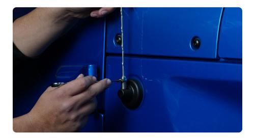
STEP 3 | Using a T40 Torx bit, remove the (4) factory bolts on each side, (8) bolts in total.
