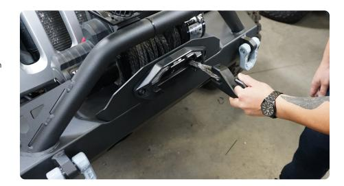
STEP 2 | Using snap-ring pliers, remove winch shackle hook snap-ring and shackle pin.
