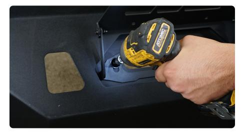
STEP 8 | Align license plate bracket with bumper and secure the provided M12 hardware using a 19mm wrench and #8 Allen bit.
