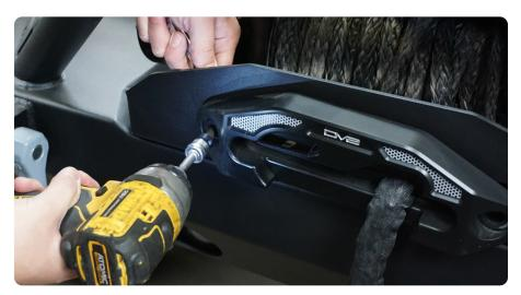
STEP 6 | Reinstall winch cable shackle hook using snap ring pliers.
