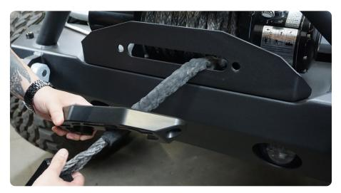
STEP 4 | Feed winch cable through license plate bracket and fairlead, install license plate bracket sandwiched between the bumper and fairlead.
