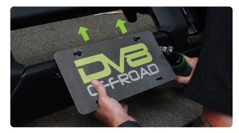
STEP 4 | Raptor owners: Use the provided spacers and M8x40mm hardware to loosely secure the bracket to the bumper. (1 spacer &1 M8 flat washer per M8x 40 Allen head bolt)
