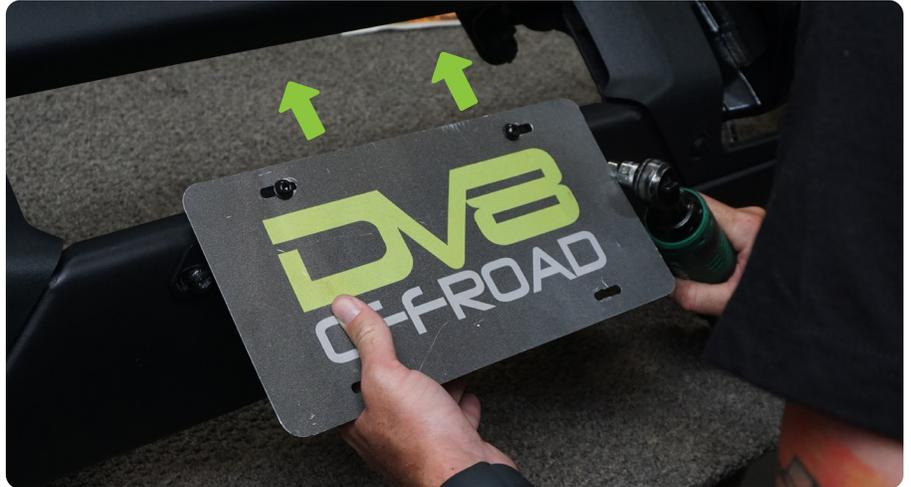
**STEP 4** | While pushing up on the license plate, secure it to the bracket using the provided M6 hardware with a 4mm allen bit and 10mm wrench.
