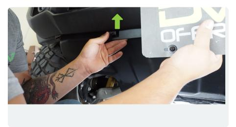
STEP 4 | When the bracket is properly installed it will rest against the factory bracket as shown here.
