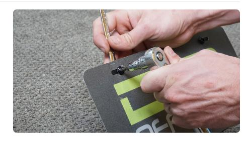
**STEP 3** Use a 13mm wrench to remove the two factory bolts located between the bumper and skid plate, directly below the two front inner sensors on the bumper.
