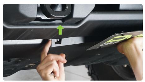
**STEP 5** When the bracket is properly installed it will rest against the factory bracket as shown here.
