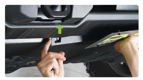
STEP 5 | When the bracket is pushed up into place, slide it to the driverside and then pull it down to seat it into place.
