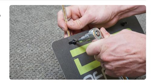
STEP 3 Use a 10mm wrench to loosen the two factory bolts located between the bumper and skid plate, directly below the two front inner sensors on the bumper.
