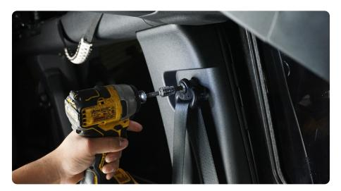
STEP 5 | Use a T50 to remove the two factory bolts securing the hardtop.
