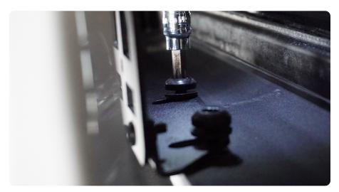
STEP 7 | Secure the mount at the seat belt by placing the spacer behind the mount and installing the seatbelt over it using a T50 and the factory bolt. Torque to with a dab of blue Loctite.
