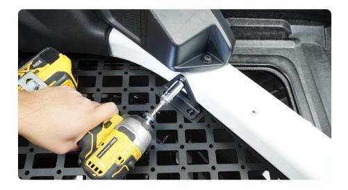
STEP 9 | Finish securing all M6 hardware using a 4mm allen bit.
