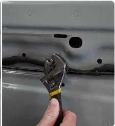
STEP 5 | Loosely install the molle panel to determine where to place the bottom four nutserts and bolt supports.
