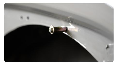
STEP 10 | Use a 12mm wrench to hold the spacer while tightening with a 10mm socket. Tighten slowly until the nutsert is set properly. Do not over tighten.
