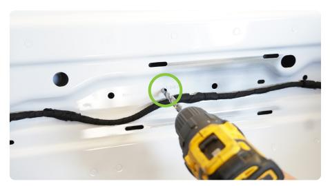
STEP 3 | Install the provided M6 nutserts using a nutsert tool, or the provided nutsert tooling kit.
