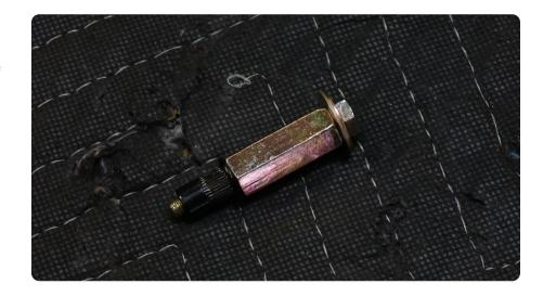
STEP 9 | Slide the nutsert tool with the nutsert into the mounting hole. Ensure the flange of the nutsert is flat against the vehicle prior to tightening.
