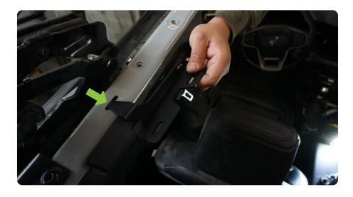
Install the provided pressure mounting plate over the provided spacers and loosely secure in place using the provided M8 hardware and a 13mm socket.
