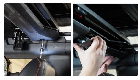
STEP 11 | Using a T40 torx tool, remove the four bolts securing the crossbar to the mounting brackets.
