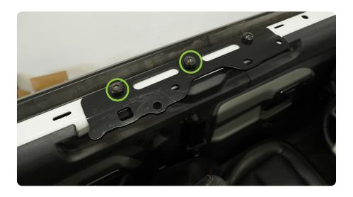
**STEP 13** Use a 8mm wrench to remove the bolt on the interior of the roll bar.
