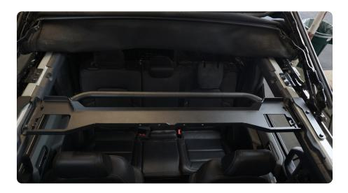
**STEP 19** Install the Molle panel, loosely secure it to the front mount and cross brace using the provided M6 hardware, #4 Allen tool and 10mm socket/ wrench.
