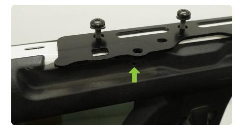
STEP 14 | Loosely Install the roll bar brackets using the factory hardware and an 8mm socket. Make sure the bracket grabs the slotted hole on top of the roll bar.
