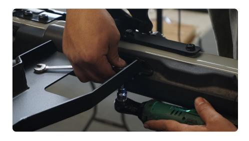
STEP 21 | Use an 8mm wrench to secure the factory hardware holding the roll bar bracket to the roll bar.
