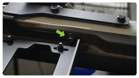
STEP 22 | For soft top models, use a 13mm socket to secure the pressure plate hardware.
