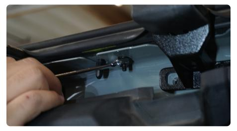
**STEP 7** I Install the front mounting bracket as shown and secure using the factory hardware with a T50 Torx bit and a 10mm wrench.
