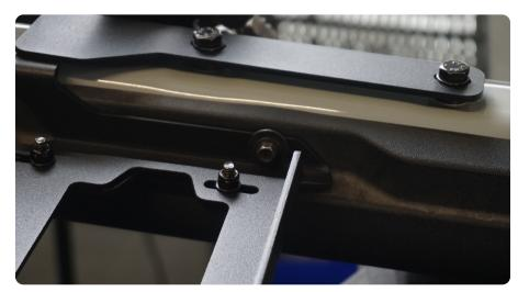
STEP 19 | Use a 13mm socket or T50 Torx bit to secure the hardware holding the mounting plate to the roll-bar.
