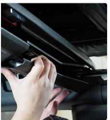
STEP 11 | Using a T40 torx tool, remove the four bolts securing the crossbar to the mounting brackets.
