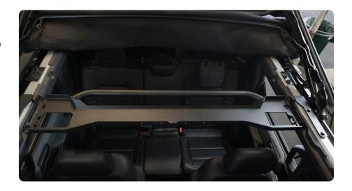
STEP 16 | Install Molle panel and loosely secure it to the front mount and cross brace using the provided M6 hardware.
