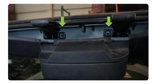
STEP 6 Use a 10mm wrench to remove the nut located between the bolts removed in step 5.
