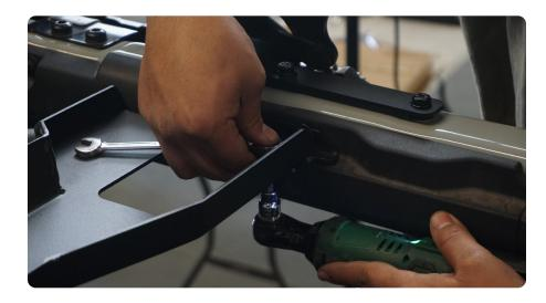
STEP 18 | Use an 8mm wrench to secure the factory hardware holding the roll bar bracket to the roll bar.
