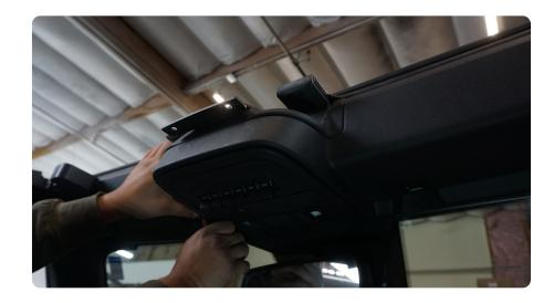
STEP 9 | Install the sun visor catches using a "L" shaped T20 Torx bit.
