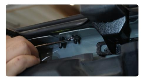
STEP 7 | Install the front mounting bracket as shown and secure using the factory hardware with a T50 Torx bit and a 10mm wrench.
