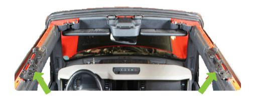
STEP 13 | Use a 8mm wrench to remove the bolt on the interior of the roll bar.
