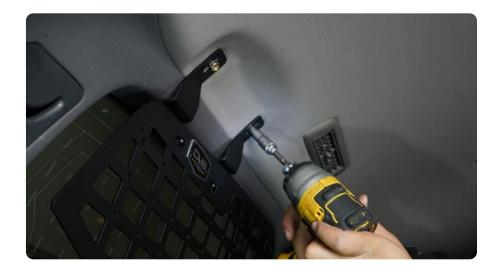
STEP 10 | Secure the bottom of the molle panel to the aluminum spacers using the M6x12 hardware (This is the shorted hardware provided) and a 4mm allen bit.
