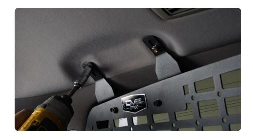
STEP 5 | Loosely install the aluminum spacers at the bottom of the molle panel using the provided M6x12 hardware (This is the shortest hardware provided). Use a 4mm allen bit if necessary.
