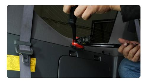
STEP 8 | Secure the aluminum spacers into the rivnuts.
