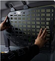
STEP 6 | Mark the mounting holes for drilling by slowly pushing the panel against the body of the vehicle and marking with sharpie where the threaded stud lands.
