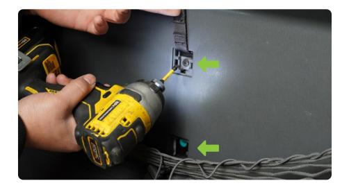
STEP 3 | Remove the factory tool kit and cover by turning the plastic handles to unlock the cover.
