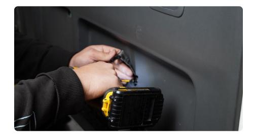
STEP 10 | Snap the plastic clips located underneath the handle into place by pressing them.
