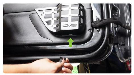
$\begin{array}{c|c} \text{STEP 3} & \text{Place the spacer between} \\ \text{the door panel and the L bracket.} \end{array}$
