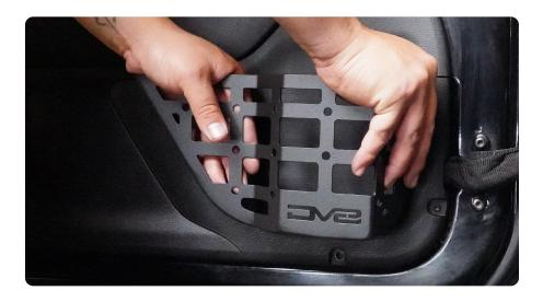
STEP 5 | Secure the pocket by inserting the provided hold down bracket into the bottom hole.
