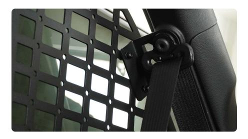
STEP 10 | Loosely secure the Molle panel to the bottom mounting bracket using (3) of the provided M6 Allen head bolts.
