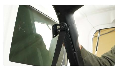
STEP 8 | Place the DV8 Pocketed Molle panel on top of the bottom mounting bracket and behind the seat belt mounted bracket.
