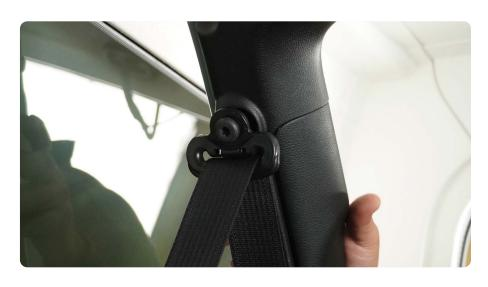
STEP 6 | Use a T50 Torx bit and an breaker bar/ratchet to break loose the seat belt bolt
