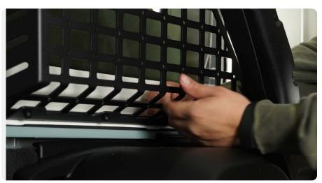
STEP 11 | Adjust the molle panel as needed, ensuring that the molle panel does not make contact with the interior trim or hardtop.
