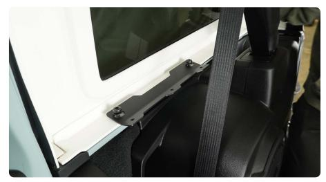
**STEP 5** | With a firm grip or using a trim clip tool, remove the seat-belts center cap by pulling straight backwards.
