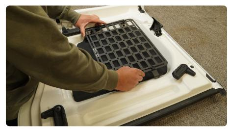
STEP 4 Using a marker, mark the holes on the mounts without letting the panel/mounts move at all.
