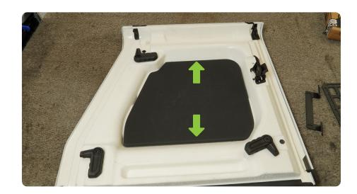
STEP 2 Using our UNMP-04, loosely mount the panel onto the brackets as shown using a mix of hardware from the UNMP-04 and the JL mounting brackets using a #4 allen and a 10mm wrench.
