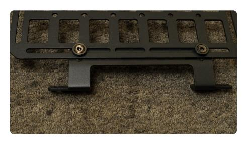
STEP 3 | Place the mount and panel onto the hardtop. Adjust the mounts so the feet with holes lay flat and the panel is in the desired position on the hardtop.
