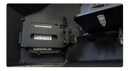
STEP 26 | Install the trailer hoist cover and trailer connector socket into the bumper by pressing each through the front of the bumper until each one is fully clicked in.
