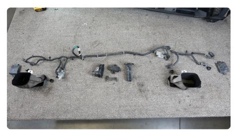
$\begin{array}{c|c} \text{STEP 15} & \text{The passenger side inner} \\ \text{parking sensors wiring loom will need to} \\ \text{be cut back to prevent the harness from} \end{array}$ pinching.
