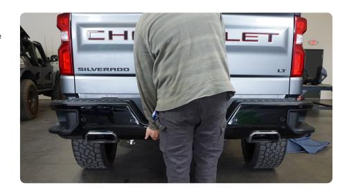
STEP 7 Using a 21mm socket, remove the bumper support upper bolts from the frame.
