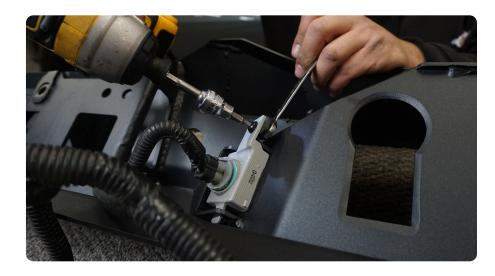
STEP 20 | Feed the factory main wiring harness through the bumper mounting brackets.
