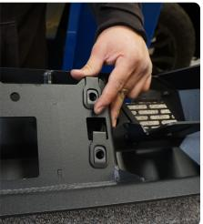
STEP 18 | If your vehicle is equipped with parking sensors, remove the parking sensor plugs from the DV8 bumper.
