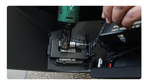
STEP 24 | Remove the 90 degree cable guide from the blind spot monitor wiring harness connector using a pick or small flathead screw driver to pry the cable guide off.
