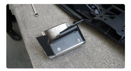
STEP 30 | Use the provided M12 Allen head hardware, an #8 Allen tool and 19mm wrench to mount the exhaust tips to the DV8 rear bumper.
