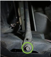
STEP 5 | Use a 18mm socket to remove the two mounting nuts (per side) that hold the OEM bumper in place.
