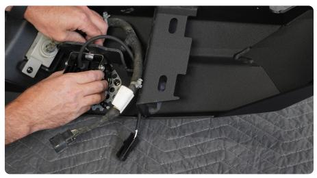
STEP 11 | Install the provided M10 clip nuts onto the bumper mounting brackets.
