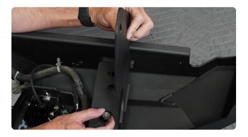
STEP 13 | With the license plate lights, trailer connector and frame brackets installed on the bumper it is ready to be mounted on the vehicle.
