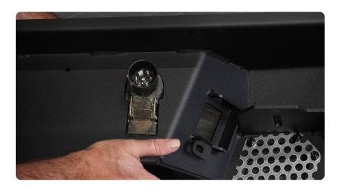
STEP 8 | Use a 10mm wrench, #4 Allen tool and the provided M6 hardware to secure the license plate light housing in place.
