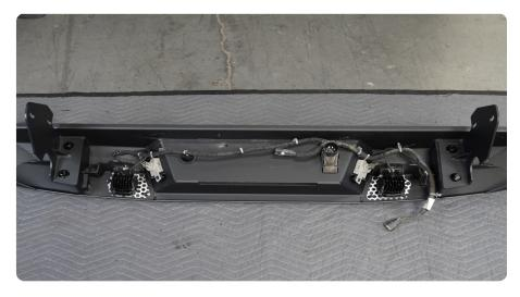
STEP 14 | With assistance lift the bumper in place and loosely secure the bumper using the factory frame bolts previously removed in step 3 and a 21mm socket.
