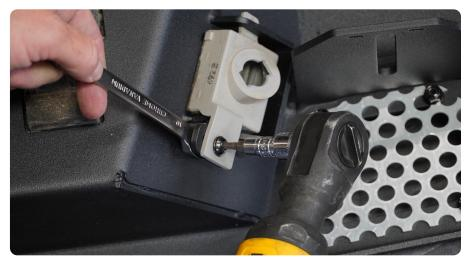
**STEP 9** | Reinstall the license plate lights in to the light housings.
