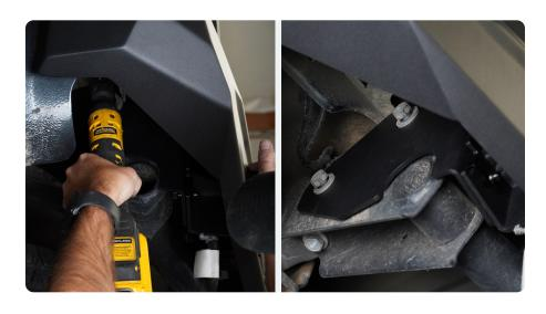
STEP 16 | Using a 16mm wrench secure hardware on the bumper mounting brackets.
