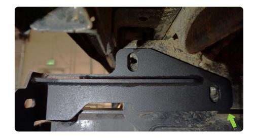
STEP 26 | The factory tow hitch/bumper support frame bracket mounting holes will need to be slightly slotted. Mark the amount of material that will need to be removed.
