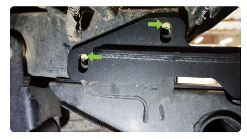
STEP 27 | Use a small sanding wheel or drill bit to remove the material and slot the mounting holes on each side.
