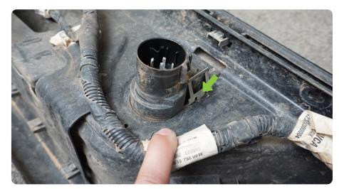
$\begin{array}{c|c} \text{STEP 11} & \text{Use a trim clip tool to} \\ \text{free the sensor/light harness from the} \\ \text{bumper.} \end{array}$
