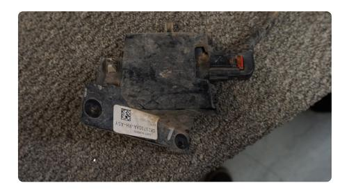
STEP 16 | Install the factory license plate lights using the provide M6 hardware and #4 allen.
