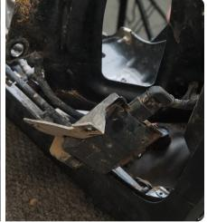
STEP 8 | Remove the back up sensors by gently prying apart the sensor bezel tabs and pressing the sensor out from the front side.
