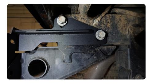
STEP 29 | With assistance, fit the bumper into place and using the M10 hardware, install the four M10 bolts per side by hand.
