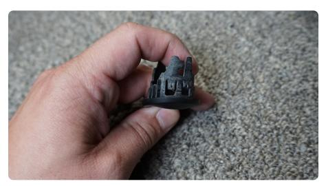
STEP 21 | Install the sensor bezel in the same position they were removed from, install the sensor into the bezel to expand the bezels locking tabs to lock the sensor and bezel in place.
