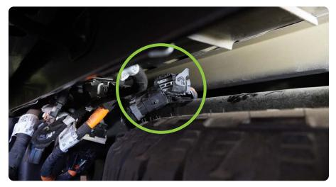
**STEP 13** Use a trim clip tool to remove any wiring harness retaining clips.
