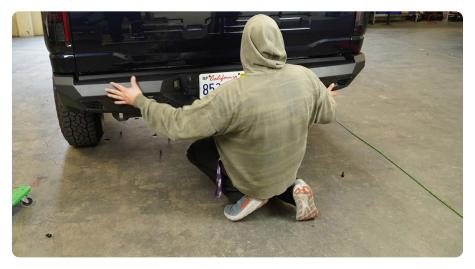
STEP 21 | Thread the provided M10x30 hex head hardware into the top mounting holes with nut clips to loosely secure the bumper to the frame.
