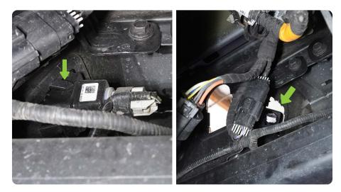
**STEP 3** Remove all parking sensor (if equipped) by spreading the sensor bezels tabs apart and pressing the sensor from the front side out the backside.
