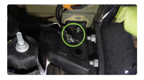
STEP 12 | Disconnect the rear parking sensor harness at the cross bar above the spare tire.
