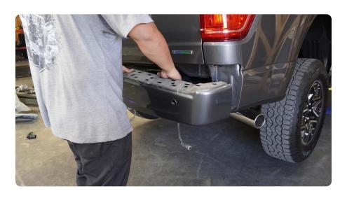
STEP 8 | Remove the hitch plate by grinding out the spot wells with your preferred grinding wheel.
