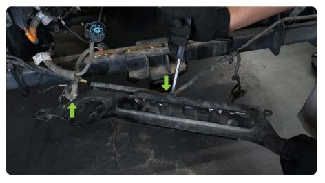
STEP 10 | Use your preferred grinding wheel to remove any left over welds from the tow hitch.
