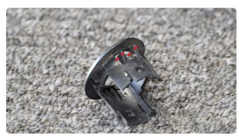
**STEP 18** | Install the sensor bezel in the same position they were removed from the factory bumper by pressing the bezel into the bumper from the front side until it clicks into place.
