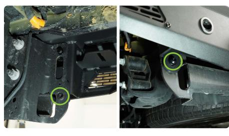
**STEP 23** Center the bumper with the vehicle and adjust the bumper up/ down as need ensuring clearance of the tailgate when close and open.
