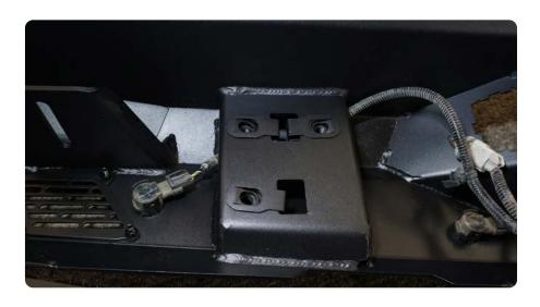
STEP 15 | Reconnect the harness to the license plate lights and install the center parking sensor into their bezels.
