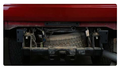
STEP 7 | Moving back to the factory rear bumper, remove the trailer plug by depressing the metal clips on each side using a trim tool.
