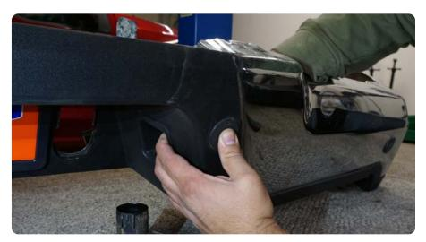
STEP 9 | With the parking sensor removed, you can remove the bezel through the face of the bumper.
