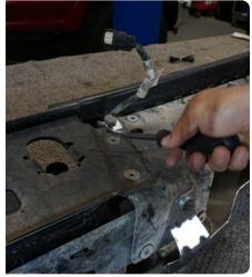
$\begin{array}{c|c} \text{STEP 12} & \text{Carefully remove the} \\ \text{electrical harness from the bumper.} \end{array}$
