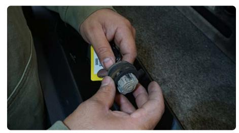
$\begin{array}{c|c} \text{STEP 18} & \text{Install the spare tire lock} \\ \text{onto the DV8 spec rear bumper.} \end{array}$
