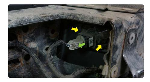
STEP 11 | Using a trim tool, remove all push pin clips that secure the bumper harness to the bumper.
