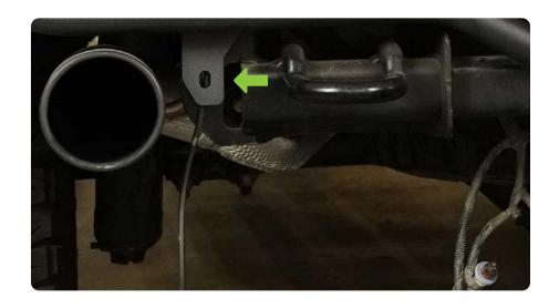
STEP 17 | Using the provided M10 hex head bolt, install the bolt into the nut clip on the backside. Secure using a 16mm socket.
