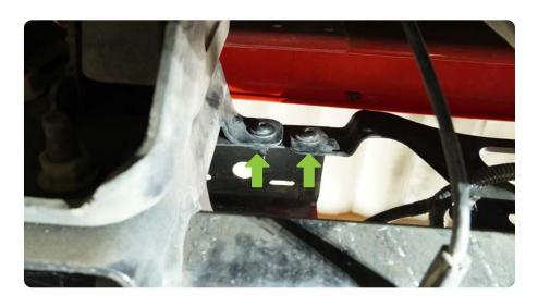
STEP 8 Using a trim tool, detach the harness from the bumper caps. Remove the caps.
