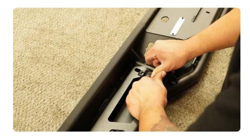
STEP 12 | Reinstall; I the license plate lights in the same direction they were removed from the factory bumper. These should lightly click into place.
