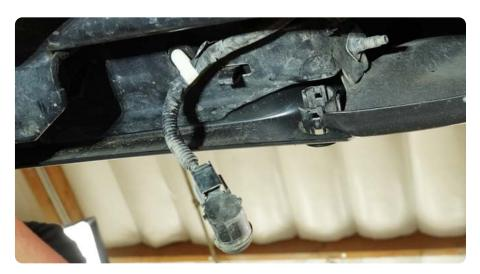
STEP 5 | From the backside, depress the two tabs on each license plate lights. Unplug the lights and set off to the side.
