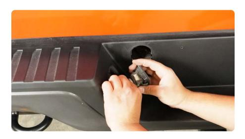
STEP 6 | While tools are not necessary, they can be used. Pry up on the plastic portion of the bumper. With pressure it should release.
