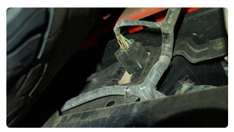
STEP 3 | With the plug pulled out, the wiring should be easy to access. Depress the plug tab and pull away from the trailer plug.
