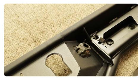
$\begin{array}{c|c} \text{STEP 13} & \text{Install the trailer plug until} \\ \text{it clicks into place.} \end{array}$
