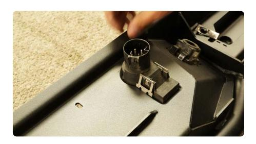
STEP 14 | Install the locking spare hoist cover into the new bumper.
