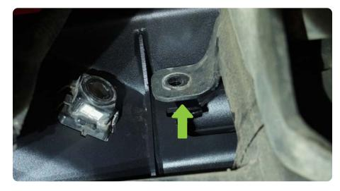
STEP 18 | Remove the sensor plugs.
