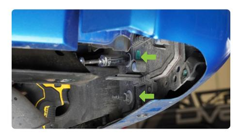
STEP 8 | If equipped with a bumper mounted hitch ball, remove this at this time.
