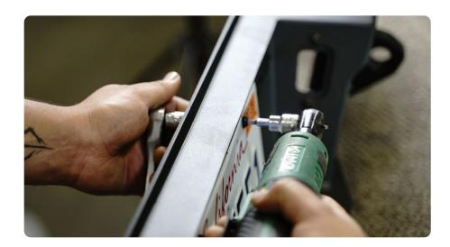
STEP 23 | Install the flat nuts onto the upper mounting hole on each side of the bumper.
