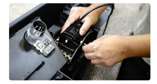
STEP 19 | If you have sensors, install the bezels on the DV8 bumper in the orientation they were removed from the factory bumper.
