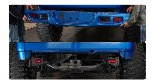
STEP 10 | If equipped with factory bed slider mounts and factory tow hooks remove both at this time.
