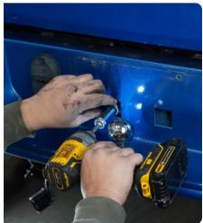
STEP 7 Using the 16mm socket, remove the four bolts ((2) on each side), holding the bumper to the hitch.
