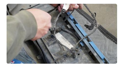
STEP 13 | Remove factory 4/7pin trailer plug by pushing in both sides of the metal clip to release the plug.
