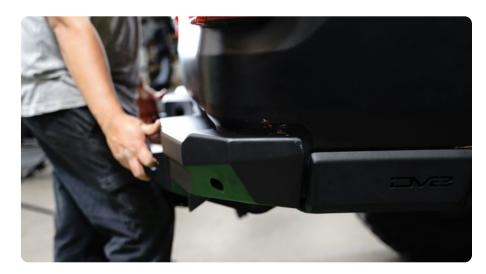
STEP 25 | Use a 16mm and 17mm socket with a 6mm allen bit to secure the hardware holding the bumper to the vehicle.
