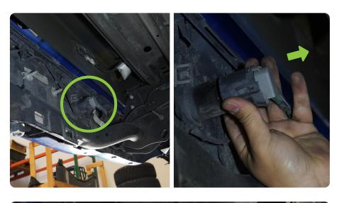
**STEP 4** At the top of the driver side frame rail, unplug the rear bumper main harness.
