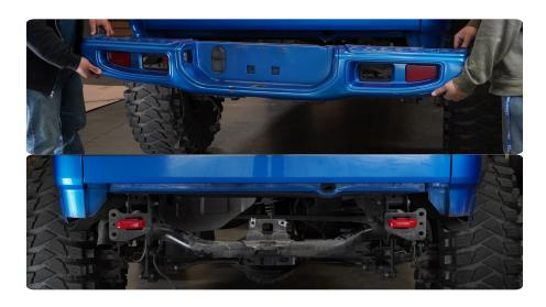
**STEP 13** | If equipped with factory bed slider mounts and factory tow hooks, use a 18mm socket to remove both items from vehicle since they cannot be used with the new bumper.
