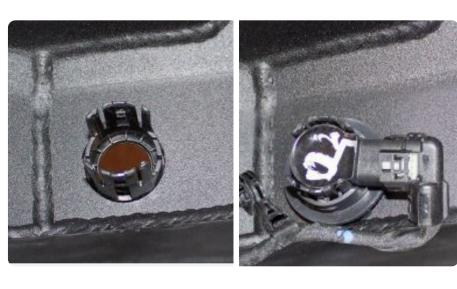
**STEP 23** | Plug in both license plate lights and install lights using hardware included with the lights (optional).
