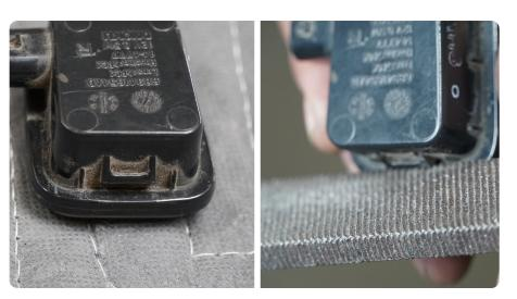
STEP 20 Once smooth, remove the license plate light mount that is install on the bumper with a #3 allen head and 10mm socket. Install the light carefully to not break off the lower tab on the light and ensure light is tight and sits flush onto bracket.
