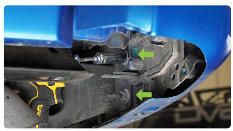
**STEP 10** | If equipped with a bumper mounted hitch ball, remove this at this time. If equipped with the factory Class III hitch, you can skip this step.
