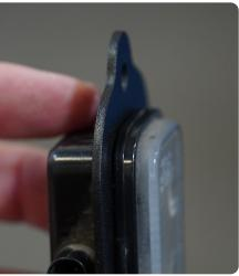
STEP 21 | Install lights into bumper. Wide part of the light should be facing up, and plug should be facing towards the back of the bumper.
