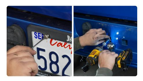
STEP 9 Using the 16mm socket, remove the four bolts (2) on each side, holding the bumper to the hitch.
