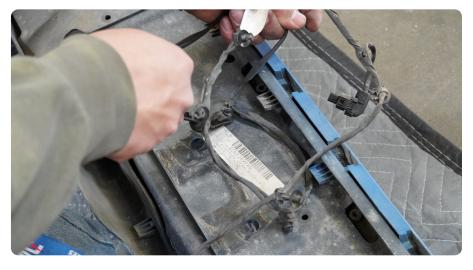
**STEP 18** | Remove factory 4/7pin trailer plug by pushing in both sides of the metal clip to release the plug.
