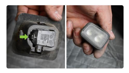
STEP 17 Using a push pin removal tool, remove the harness from the bumper. The amount of pins will vary depending on if equipped with sensors or not.
