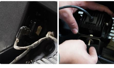
STEP 24 | If equipped, install the trailer plug into provided bracket. Using the provided M8 hardware, mount plug into bumper ensuring plug is facing down.
