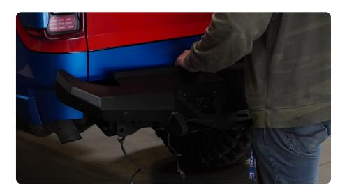
STEP 26 Using the M12 allen head bolt on the bottom, install hardware using a #8 allen head and 18mm socket.
