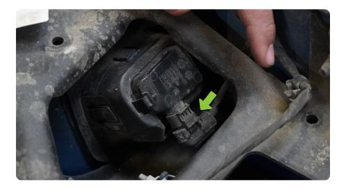
STEP 15 | There are four tabs on the outside of the license plate light. Three of four need to be lifted for light to be removed. Once three of the four tabs are pulled back like shown, push the light towards the face of the bumper to remove.
