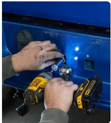
STEP 9 | If equipped with a bumper mounted hitch ball, remove this at this time.
