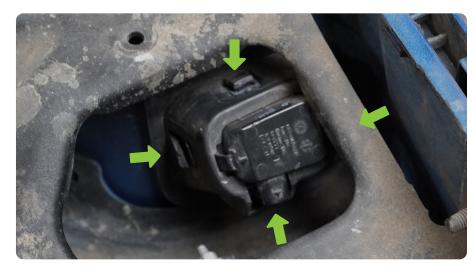
STEP 22 | Push on tap to release light from housing.
