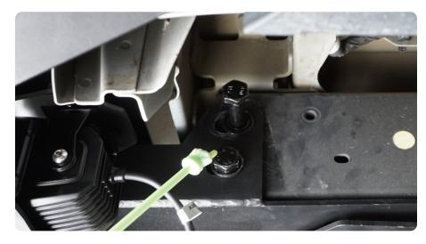
STEP 27 | Adjust the in-out position of the bumper/hitch and secure all (4) provided M14 hardware using a 21mm socket and 22mm wrench.
