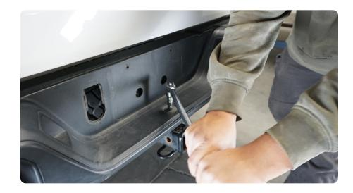
STEP 16 Use a 21mm socket with a 22mm wrench to remove the harwdare securing the hitch to the vehicle. Use assistance to support the hitch while the hardware is being removed.
