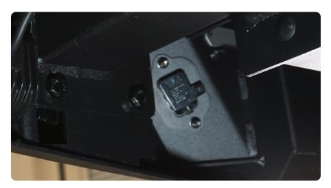
STEP 25 Using a #4 allen bit and the provided M6 hardware, install the license plate holder.
