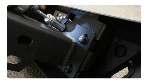
STEP 19 | Using a 10mm wrench, #4 allen bit and the provided M6 hardware, attach the trailer plug mount (if equipped).
