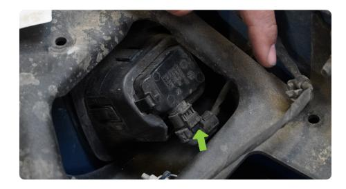
STEP 21 | There are four tabs on the outside of the license plate light. Three of four need to be lifted for light to be removed.
