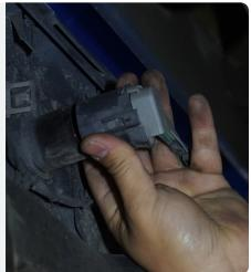
$\begin{array}{c|c} \text{STEP 4} & \text{At the top of the driver side} \\ \text{frame rail is the main bumper harness.} \end{array}$
