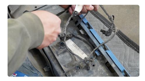
STEP 14 | Remove factory 4/7pin trailer plug by pushing in both sides of the metal clip to release the plug.
