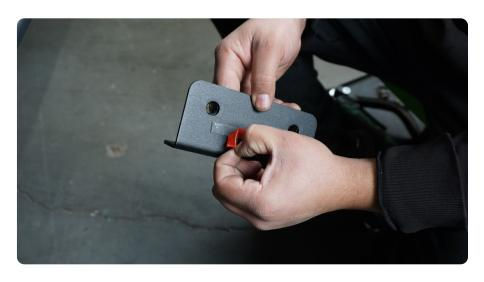
**STEP 10** | Insert and position the nut plate so it is lined up with the existing holes in the sides of the frame rail.
