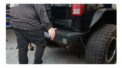
**STEP 11** With the bumper mounts loosely secured to the frame, adjust the side to side/up and down position of the bumper until it is in the desired position.
