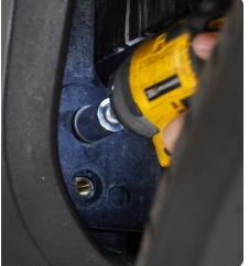
STEP 5 Use a 16mm socket to remove the remaining four bolts securing the bumper to the vehicle located between the bumper and rearmost body mount.
