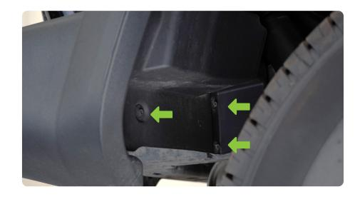
STEP 4 Use a 16mm socket to remove the bolts securing the bumper brackets to the bumper. These are located on the edges of the bumper behind the rear tires.
