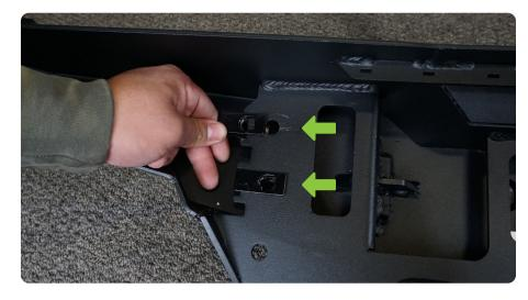
STEP 10 | Loosely secure the mounts onto the bumper using the provided M12 hardware.
