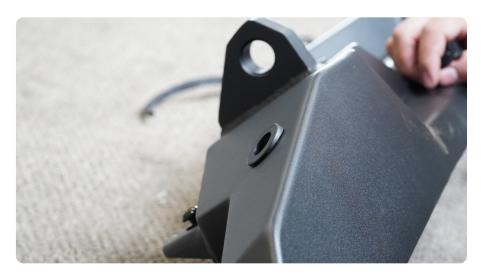
STEP 12 | With the bezels in place, run the sensor wiring harness though cavity in the bumper aligning the sensors with the bezels. Push Sensors into bezels ensure they have "clicked" into place. Secure sensor harness using provided zip tie tabs.
