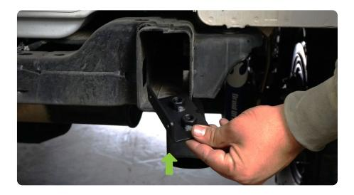
STEP 9 | Install the flat nuts into the top two mounting holes on each side of the bumper by pressing them into place.
