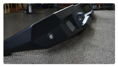
**STEP 9** With the bezels in place, run the sensor wiring harness though cavity in the bumper aligning the sensors with the bezels. Push Sensors into bezels ensure they have "clicked" into place. Secure sensor harness using provided zip tie tabs.
