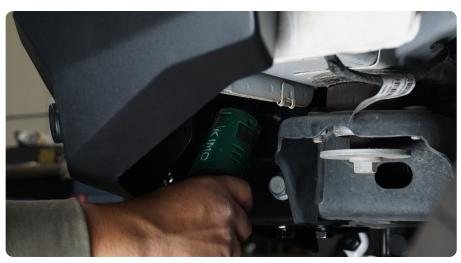
STEP 22 | Adjust the in-and-out position of the bumper ensuring there are consistent gaps between the bumper and vehicle, and that the bumper is not touching the vehicle.
