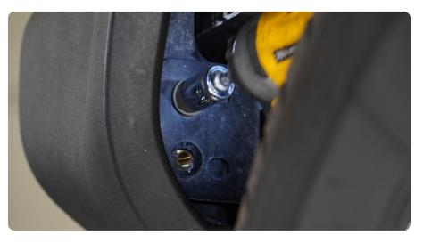
**STEP 5** Use a 16mm socket to remove the remaining four bolts securing the bumper to the vehicle located between the bumper and rearmost body mount.
