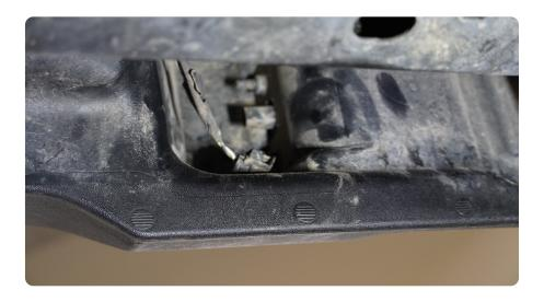
STEP 2 Disconnect the bumper wiring harness using a panel clip tool or flat screwdriver to pry open the white locking clip and remove.
