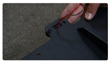
STEP 16 | To connect the license plate light, cut off the factory license plate light plug and either cut back the factory wire loom to expose more wire length, or use 22g wire to extend the harness.
