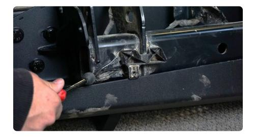
STEP 32 | Secure the hitch to the mounting brackets using the M10 hardware with a 16mm wrench and socket.
