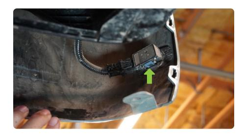
STEP 8 | Use a trim clip tool to remove the clips securing the wiring harness, and gently pull the wiring out to prepare for bumper removal.
