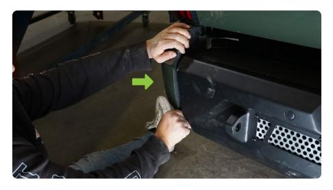
STEP 37 | Install the factory push clips running along the bottom lip of both fenders.
