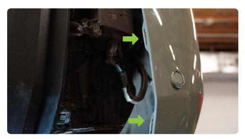
STEP 6 | Unplug the wiring harness located behind the trim on the passenger side of the vehicle.
