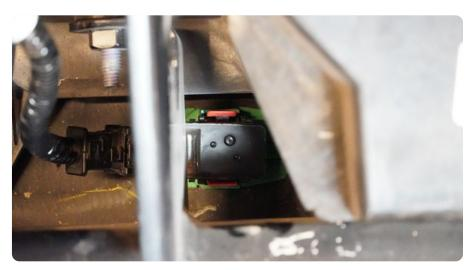
STEP 12 | Use a 10mm socket to remove the bolt securing the proximity sensor.
