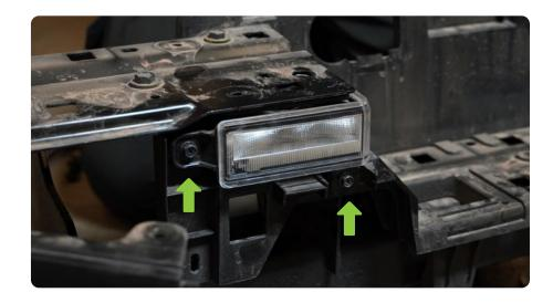
STEP 20 | Use a 12mm socket to remove the bolts on the hitch step and two top sections securing the trim to the hitch.
