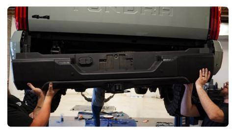
STEP 10 | Use a trim clip tool to remove the clips securing the sensor wiring harness to bumper and set it off the to side for installation on the DV8 bumper.
