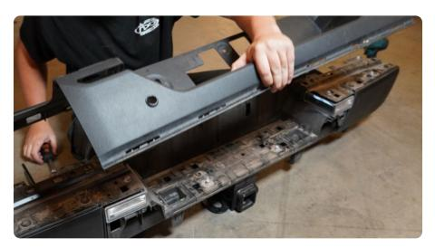
STEP 18 | Use a trim clip tool to remove the clips securing the remaining trim pieces to the bumper.
