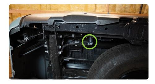
STEP 2 | Unplug the three wiring harnesses located next to the spare tire on the passenger side using a trim clip tool to press the release tabs and pull.
