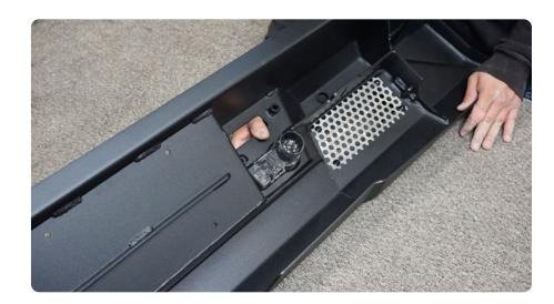
STEP 23 | If you are installing pod lights on the bumper, do so at this time using the hardware provided with the lights.
