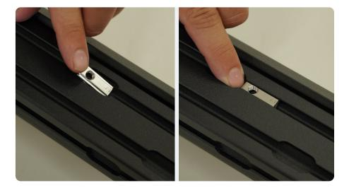
STEP 10 | Align the T-nuts with the side rails upper counter sunk mounting holes, use the provided M6x12mm counter sunk hardware to secure the side rail to the cross bar on each side at the front and rear.
