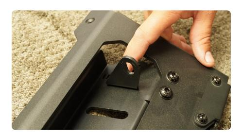
STEP 28 | Mount the front light bar plate with lip to the front of the roof rack, ensure that this plate is between the side rails.
