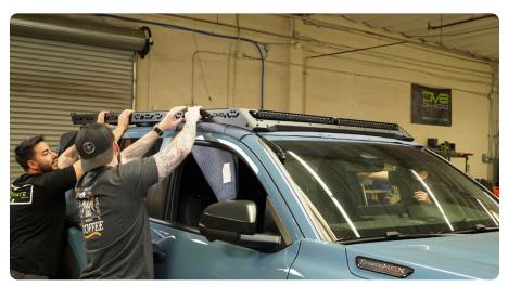
STEP 21 | Install all M8 Mounting bracket hardware by hand.
