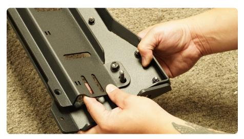
STEP 27 | Mount the light bar brackets. These bracket will allow you to run two 20" LED Light Bars.
