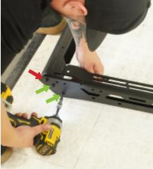
STEP 4 Use the provided M6x30mm allen head bolts and a #4 allen tool to loosely attach the middle and front cross bars to the side rails.
