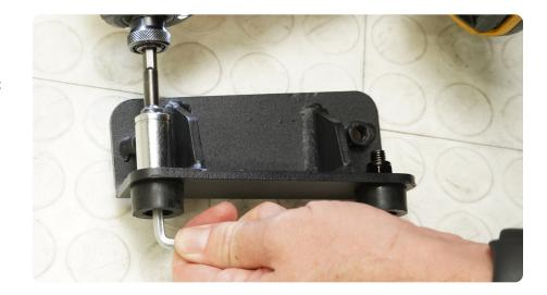
STEP 15 Using a #4 allen tool and the provided M6 hardware, mount the front bracket to the inside of the roof rack rails.
