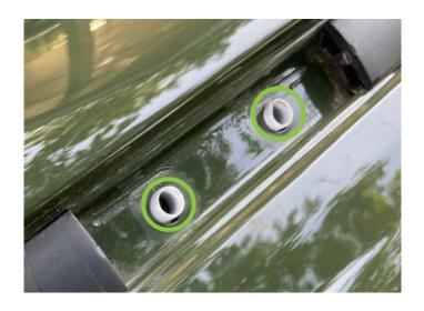
STEP 18 | Using a #5 allen tool, turn the threaded bolt down until you feel slight resistance.
