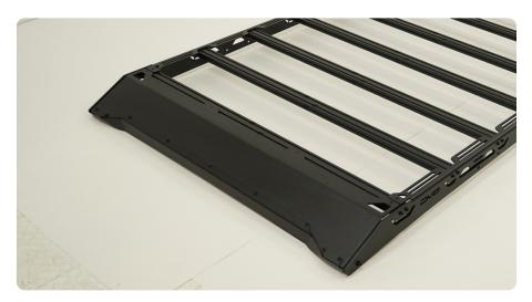
STEP 13 | Using the provided blue thread locker, assemble the roof mounting hardware and provided spacers together, ensuring an equal amount of threads is on each side of the spacer.
