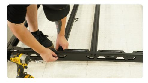
STEP 7 Using the provided M6x20mm allen head hardware, a #4 allen tool and 10mm wrench, secure the front lip to the wind deflector plate.
