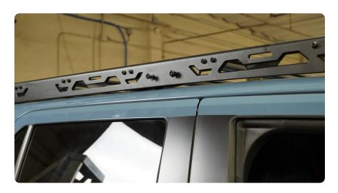
STEP 22 | With all M8 mounting bracket hardware loosely started, secure the M8 hardware using a #5 allen tool.
