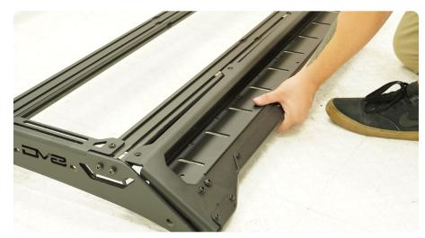
STEP 29 | Using the provided M8 hardware, a #5 allen tool and a 13mm wrench secure the front of the fascia plate to the side rails.
