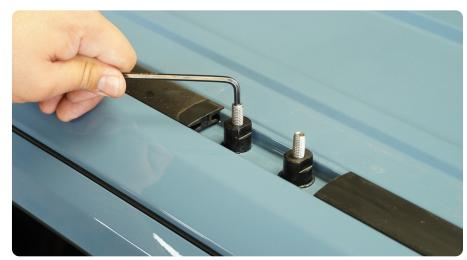
STEP 19 | Loosely secure the bracket to the spacers previously installed. The M8 nylon nuts should but just tight enough that you are still able to adjust the brackets in and out, with a firm grip.
