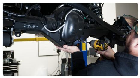
STEP 7 | Hold down the swaybar over the mounting holes, and thread the longest M8x40 hardware through the top mounting hole.
