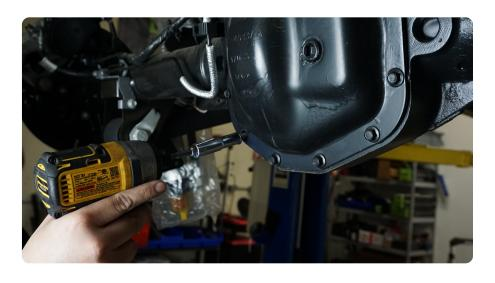
STEP 6 | Slide the nut plate behind the track bar mount and use the notches on the nut plate to allow it to rest in place.
