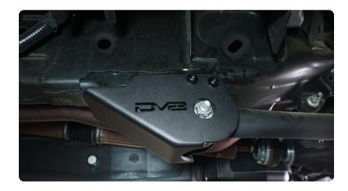
STEP 9 | Passenger side installation ---(Plastic fuel tank skid plate equipped): Using the provided T25 Torx key remove the (2) factory torx screws and plate.
