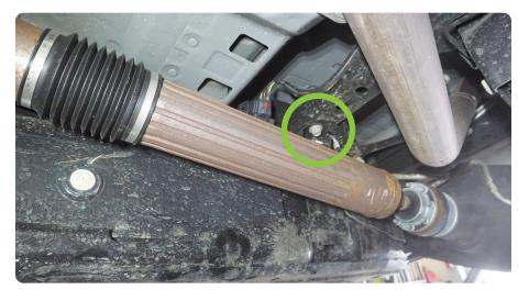
STEP 11 | Use an 18mm socket to remove (3) bolts along the passenger frame rail and (2) bolts securing the skid plate to the front cross member.
