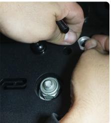
STEP 6 | Slide the provided Nut Plate behind the factory trailing arm mount.
