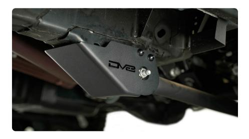
STEP 18 | Double check at all hardware is secured and both torsion bar nuts are torqued to 159FT-LBS.
