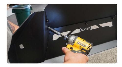
STEP 7 | With assistance loosely secure the skid plate using the provided M10 hardware.
