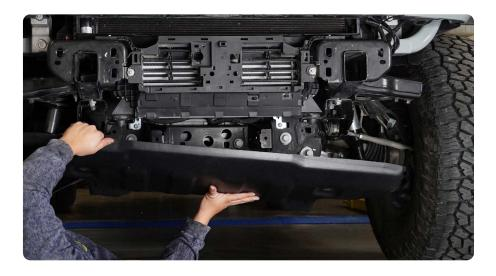
STEP 3 | With the underside exposed remove the factory bolt using a 18mm socket.
