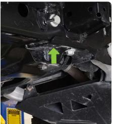
STEP 4 | Begin the assembly of the DV8 Skid Plate using the provided M8 hardware.
