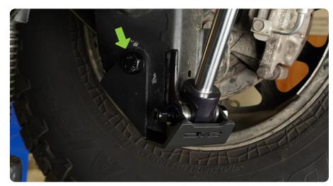
STEP 4 | Torque the M14 link bolt sing a 21 and 22mm socket/wrench and M12 shock bolt sing a 18 and 19mm socket/wrench to factory specs.
