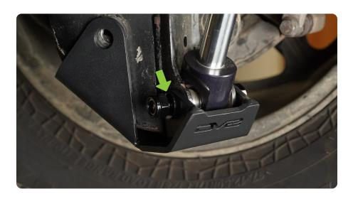
STEP 3 | Thread the provided M14 hex bolt through the skid plate and rear link.
