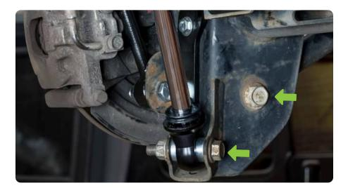
STEP 2 | Place the DV8 shock/link skid plate under the factory lower shock mount/link mount as shown.
