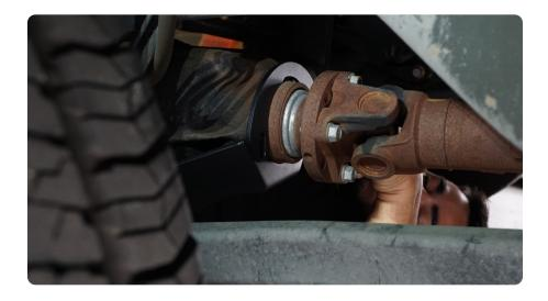
STEP 4 Using the provided M10 hardware and a 16mm socket, secure the pinon strap to the diff skid plate.
