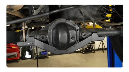
$\begin{array}{c|c} \text{STEP 3} & \text{Place the provided "U-strap"} \\ \text{over the axle as shown.} \end{array}$
