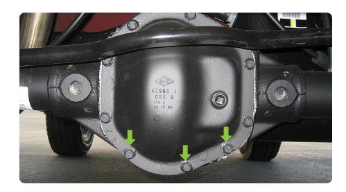
STEP 2 | Lift the DV8 D44 rear diff skid up to the rear differential, loosely secure the DV8 diff skid plate in place using a 13mm socket and the provided 5/16 flange bolts
