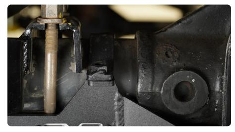
STEP 4 Using the provided M10 hardware and a 16mm socket, secure the U-strap to the diff skid plate.
