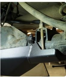
STEP 5 | Torque the three lower diff cover bolts to 24 ft-lbs.
