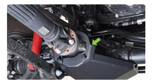
**STEP 4** While lifting up on the diff skid plate, Use a 16mm socket to secure the rear mounting bracket in place.
