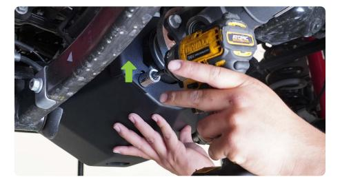
STEP 5 Use a 10mm socket to secure the (4) diff cover bolts.
