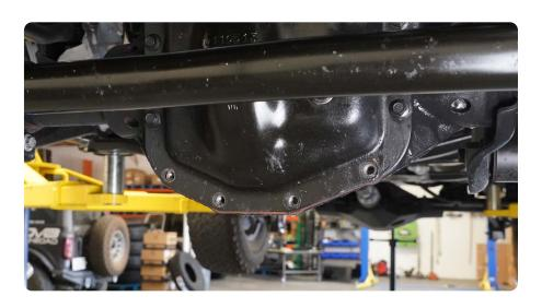
STEP 2 | Hold the DV8 Diff Skid Plate up to the bottom of the front diff and loosely install the (4) factory diff cover bolts.
