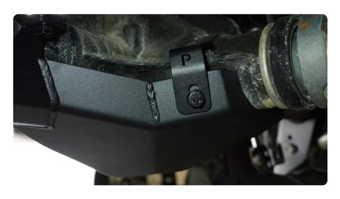
**STEP 6** With all hardware attached, push upwards on the skid plate and tighten all hardware down using a 16mm socket on the provided M10 hardware and a 10mm on the factory diff bolts.
