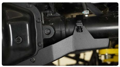
STEP 5 Using the M10 hardware loosely attach the labeled straps to the pinon. "P" for passenger and "D" for driver.
