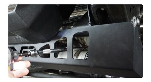
$\begin{array}{c|c} \text{STEP } 11 & \text{Double Check fitment} \\ \text{and all hardware is secure.} \end{array}$
