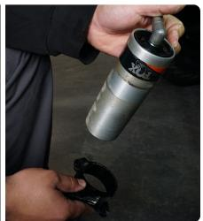
STEP 3 | Remove the lower frame cap using a 16mm socket to remove both factory bolts.
