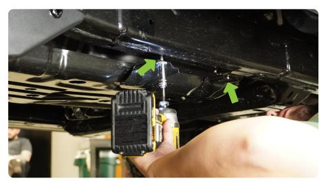
STEP 5 | With the fuel take skid plate lowered, install the provided M12 bolts into the upper mounting hole of the skid plate and though the trailing arm mount.
