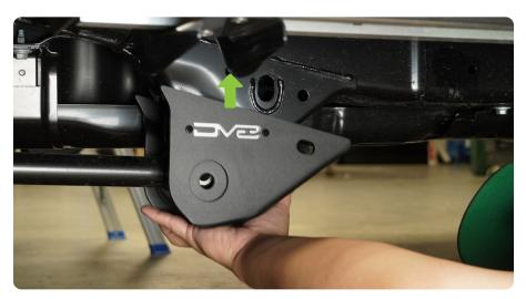
STEP 3 | With the skid plate in position loosely secure the skid plate using the factory hardware. Thread the factory nut on by hand as much as possible.
