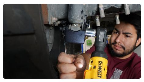
**STEP 5** | Torque both M12 bolts to 93ft lbs.
