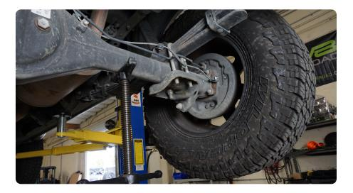
STEP 2 Use a 19mm socket to remove the (4) leaf spring U-bolt nuts.
