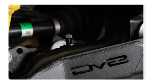
STEP 6 | Use the M10x85 bolt and loosely secure with washer and nut.
