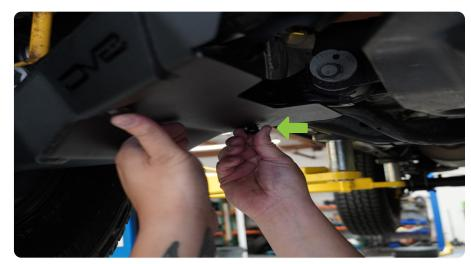
STEP 7 | Use the M6x75 bolt loosely secure with the M6 washer and nut.
