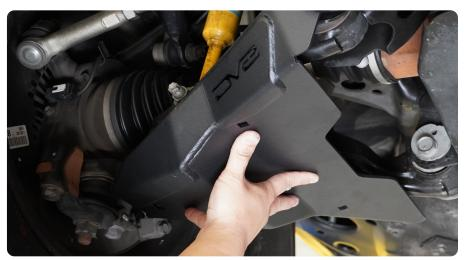
STEP 4 | Align the holes. Place carriage bolt into the skid plate pushing through the arm.
