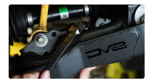
STEP 9 | Repeat on the other side. Check all hardware is secure and not touching any component of the suspension.
